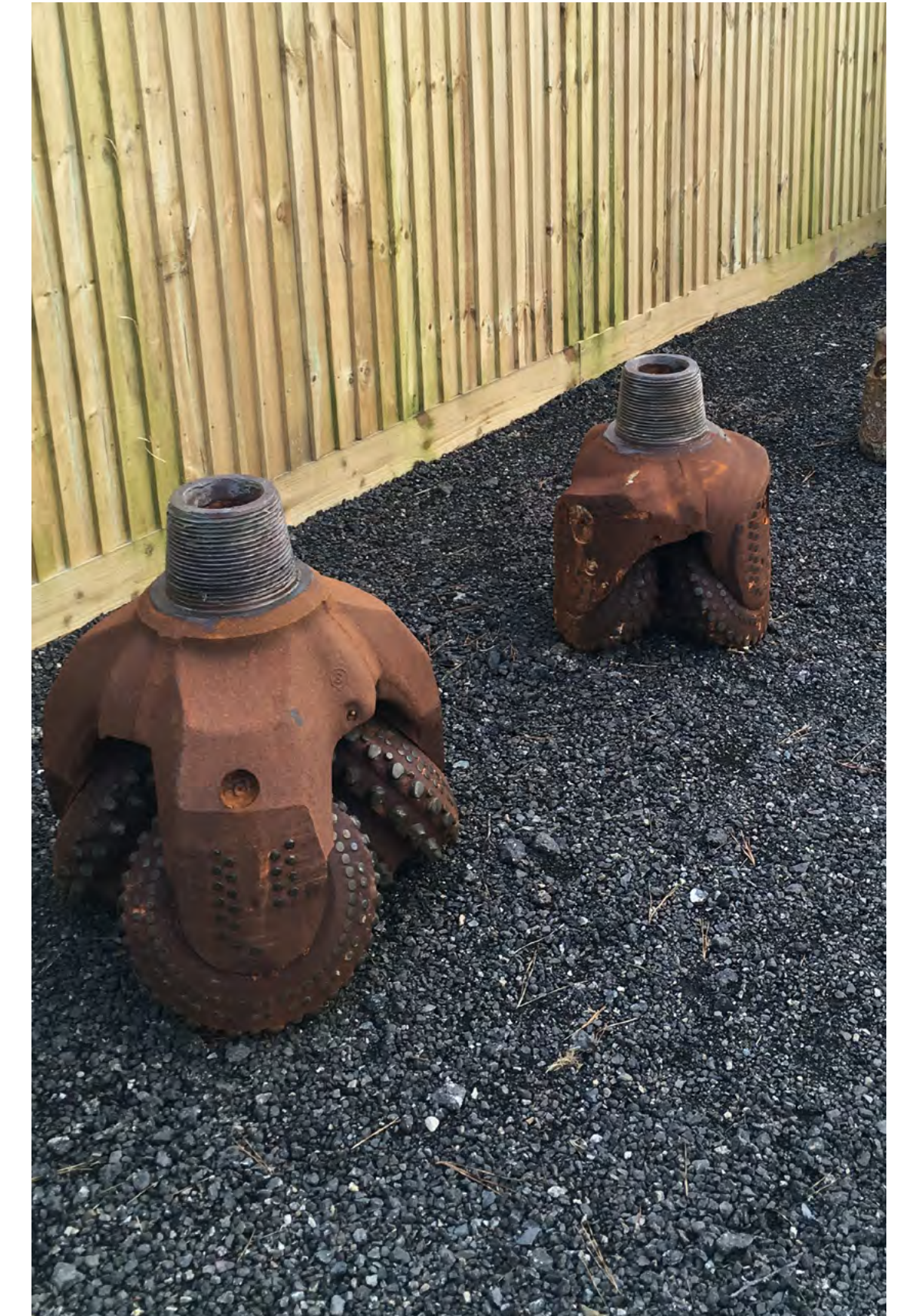
Steel tri-cone drill bits with tungsten carbide inserts used for drilling the United Downs boreholes
